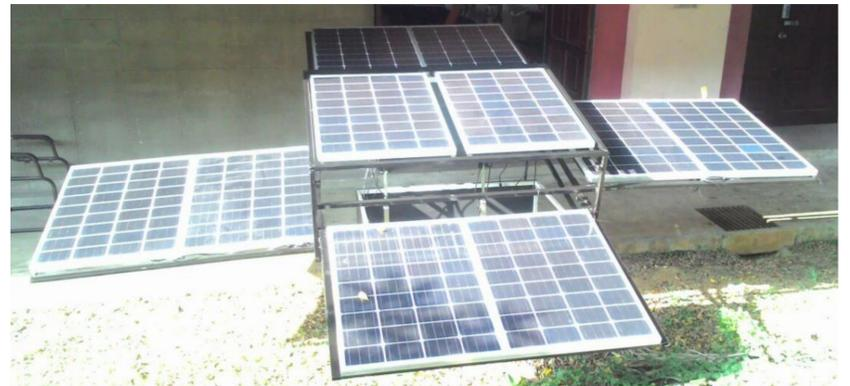
Optimized Tilted Angle Solar Modules (1kW)
